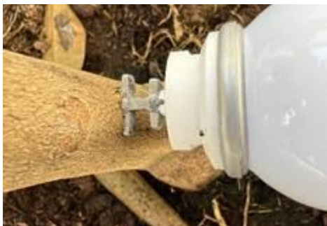
Figure 7. Over-insertion of the tip into the tree.
