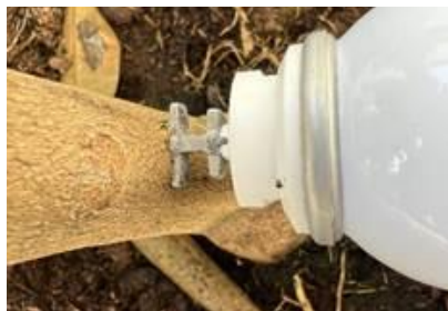
Figure 4. Over-insertion of the tip into the tree.
